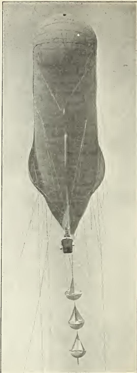
Fig. 25. Head-On View of Modern Kite Balloon,
