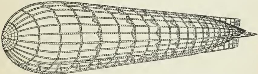
Fig. 18. Aluminum Frame Construction of Zeppelin Hull
