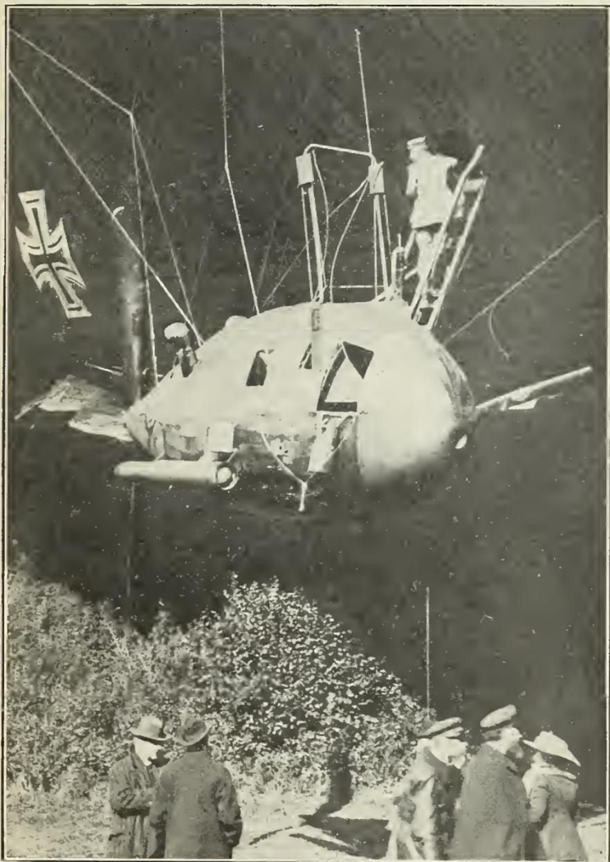
Fig. 24. One of Six Gondolas, or Power Units of the Zeppelin L-49
