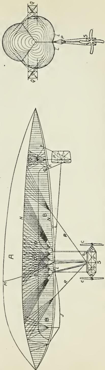
Fig. 21. Side and End Views of British Astra-Torres Dirigible Used for Anti-Submarine Patrol Service
